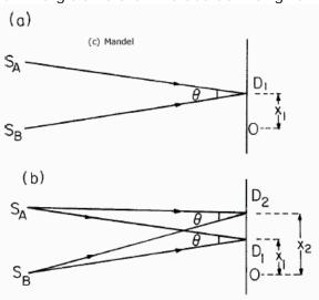
FIG. 1. Principle of photon interference: (a) one-photon or second-order interference; (b) two-photon or fourth-order interference.  $S_A$  and  $S_B$  are sources.  $D_1$  and  $D_2$  are photodetectors.
